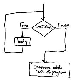
We first enter this diagram from the top. If the condition evaluates to False, then we skip the loop entirely and move on, but if it is True, we enter the body of the loop. The difference from a regular conditional is that if we do execute the body, then once we are done, we jump back and check the condition again (instead of moving on). If the condition is again True, we'll enter the loop again, and so on.
